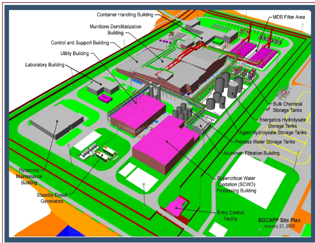
The latest overall site plan for the BGCAPP, dated January 21, 2005. The plan is subject to change with redesigning efforts to lower the cost of the overall demilitarization of the chemical weapons.
